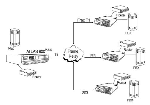
Figure 1-2. Frame Relay Circuit
